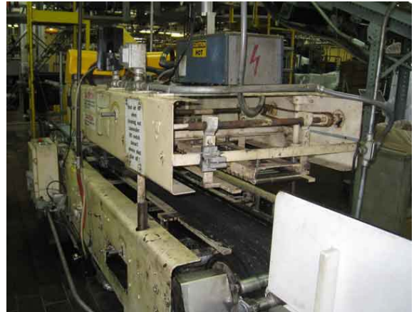
J293 CASE SEALER: Case sealer, adjustable, hot melt top seal only. Includes Nordson hot melt unit with 2 heads.
