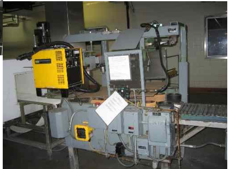
Case Sealer: Wilkins case sealer, top hot melt sealing. Model 48, serial 1032. Has Slautterback hot melt unit.
