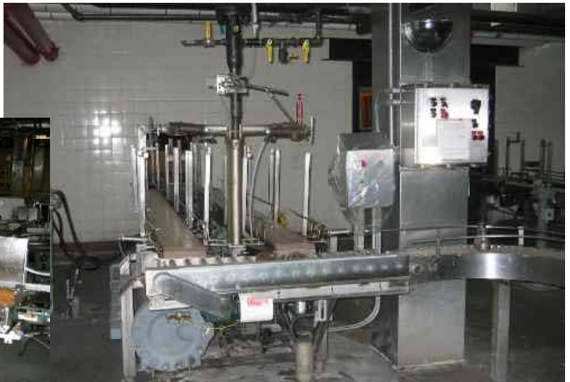
Filler: Cherry Burrell volumetric dual head filler - used for viscous materials such as shortening or margarine. Has single cylinder 12 in dia x 48 in long. Automatic operation, load cells. Also has hydraulic actuator for volume adjustment.
