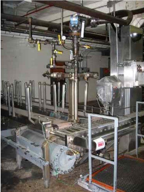
Filler: Cherry Burrell volumetric dual head filler - used for viscous materials such as shortening or margarine. Has single cylinder 12 in dia x 48 in long. Automatic operation, load cells. Also has hydraulic actuator for volume adjustment.
