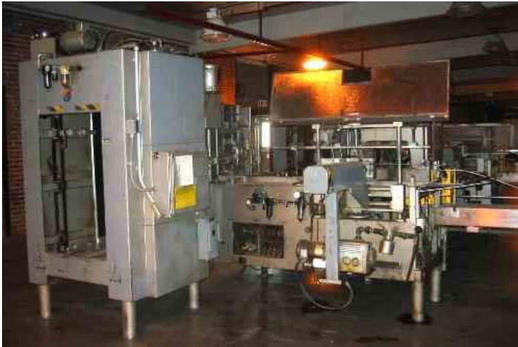
Case Erector: ABC case erector Model K1800, serial 19974. Has large magazine, serial 19975. Slautterback hot melt unit for bottom sealing.
