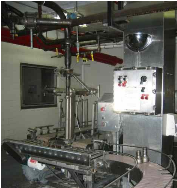
Case Sealer: Wilkins case sealer, top hot melt sealing. Model 48, serial 1032. Has Slautterback hot melt unit.
